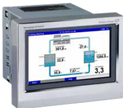
Panel version with "7" TFT display and touch control
