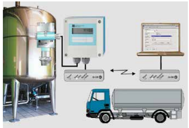
Molasses level measurement in customer specific tanks of a supplier. The Minilog B stores the customer usage and informs the supplier of the actual level in the storage tank. The data is collected at a central supply point and is available for the planning of just in time delivery.
