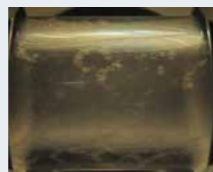
80% 蒸汽干度( x = 0.8 ) 20% 冷凝水(环流) → 报警 \triangle
