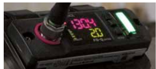
In addition to the display in the temperature control unit: Display of the flow rate and the status on the sensor
