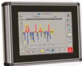
Visualization of the external temperature control circuits on a touchscreen (10,4")
