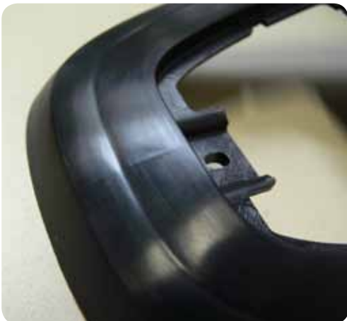
Conventional temperature control with visible weld-lines
