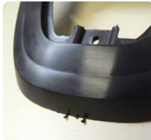
Dynamic temperature control without visible weld-lines
