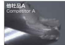
他社品A Competitor A 4穴で折損 Breakage after 4th hole
