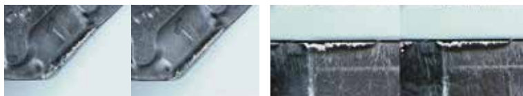
主切削刃部磨损 Wear on main cutting edge
