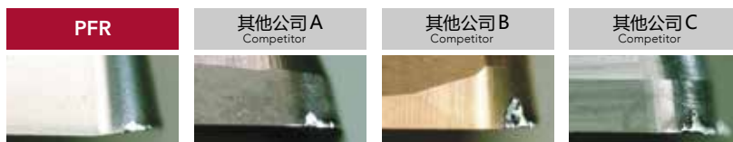
加工32.9m 时的磨损情况 State of damage after 32.9m of machining
