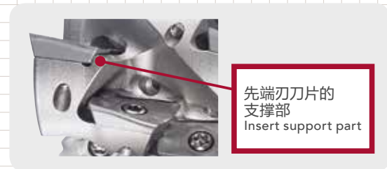
第二段以后: 重视锋利性的排列 2nd and subsequent steps: for high sharpness
