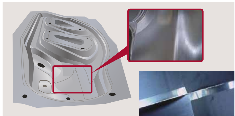
加工51小时后的刃尖状态 Cutting edge after 51 hours of milling
