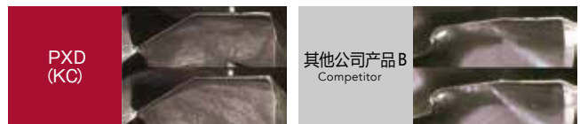
[FCD600] 加工1,600孔时的磨损比较 Wear comparison after 1,600 holes of drilling
