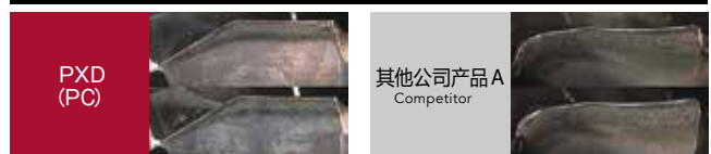
加工1,000孔时的磨损比较 Wear comparison after 1,000 holes of drilling
