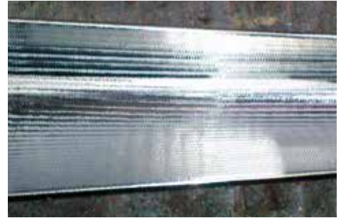
加工1,248分钟后的刃尖状态 Cutting edge after 1,248 minutes of milling.
