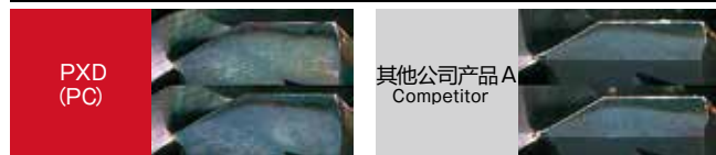
加工900孔时的磨损比较 Wear comparison after 900 holes of drilling
