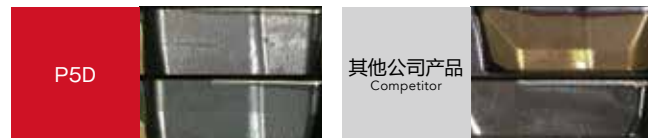
加工150孔时的磨损比较 Wear comparison after 150 holes of drilling
