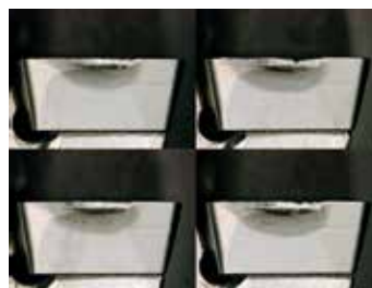
PHC (13.2m 加工时) After 13.2m of milling
