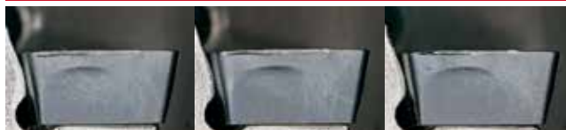
PHC 900m加工时的照片 After 900m of milling
