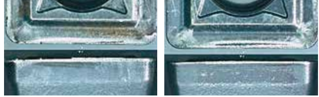
刀片磨损情况的照片(加工5个孔时) Photo of insert wear width (after 5 holes)
