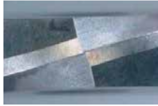
加工1,248分钟后的刃尖状态 Cutting edge after 1,248 minutes of milling.
