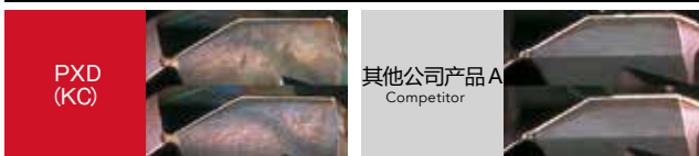
[FC250] 加工1,280孔时的磨损比较 Wear comparison after 1,280 holes of drilling
