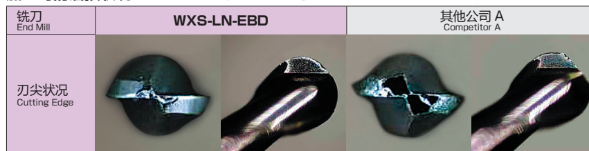
加工时的磨损状况 Tool wear after pocket milling
