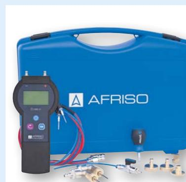
**Application** For differential pressure measurement and flow rate adjustment in heating and refrigerating systems during hydraulic balancing. To be used in conjunction with VarioQ thermostat valves and combination blocks. If VarioQ valves are used, hydraulic balancing can be done directly at the radiator. It is neither necessary to know the pipeline system nor to perform complex calculations.
