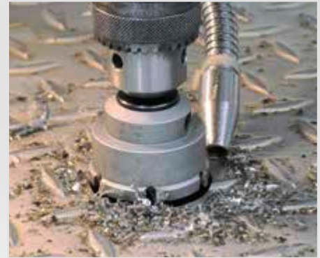
Drilling in checker sheet
