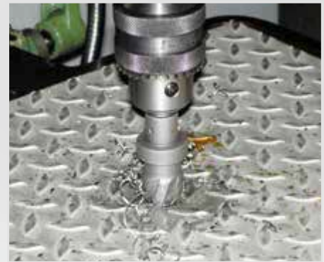
Drilling structured sheet metals
