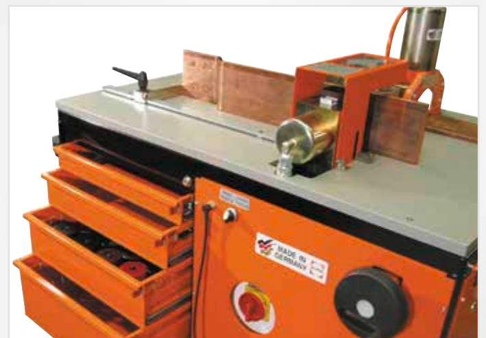
4 tool draws with compartments for punchers and dies are fitted to the trolley.
