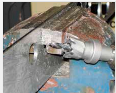
Free-hand drilling up to Ø 30 mm
