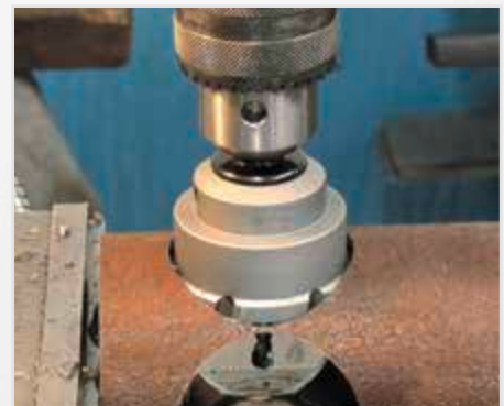
Drilling in pipes
