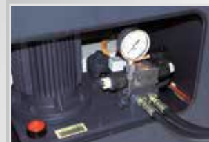
Dual-circuit hydraulic unit in cabinet base
