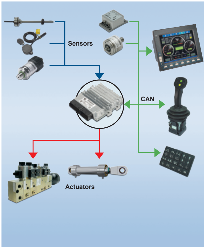
Figure 19: Centralised structure using a controller
