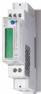
The single-phase version bi-directional energy meters is for direct current connection up to 40 A and in addition to energy, measures and transmits via the communications port other key electrical parameters for instance as voltage, current, active power, power factor, frequency...
