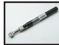
01-506, W1-7 mm Fixed break over torque wrench: 7 mm opening for W1-105x Sparkplug installation. Torque is 0.56 N*m (5 in-lbs)
